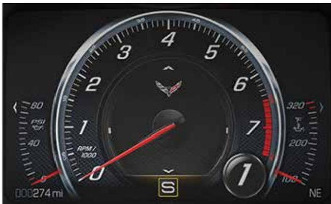
The Sport Display Theme features a circular tachometer with the DIC contained within the tachometer ring.
