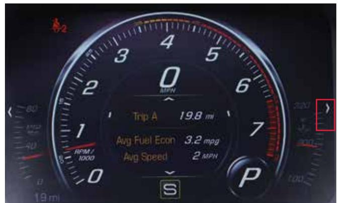
When a submenu exists in the DIC, a carat mark will point to the right. Use the right arrow on the 5-way controller to access the submenu.
