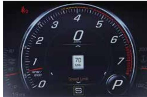
“Posted speed limit” is only available with the optional MyLink with Navigation because the information it displays comes from a database in the onboard nav system.
