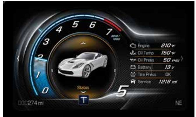
The Touring Display Theme features a partial tachometer ring containing the DIC. The area in the center is for displaying icons, Turn-by-Turn directions, maps (for vehicles equipped with Navigation), images or phone contacts.
