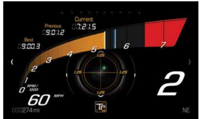
The Track Display Theme has a tachometer with prominent redline markers and three lap timers. Track theme is similar to the electronic gauges used in the C6R race car.
