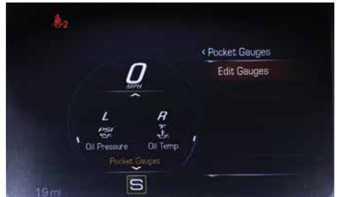
After selecting "Pocket Gauges," you can edit them, using the 5-way controller and the Edit Gauges submenu and following on-screen directions. You can choose the gauge position—right or left—and select from five gauges:
