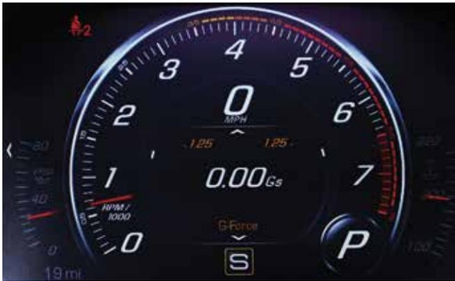
The Friction Bubble is simply a circle that displays lateral and longitudinal G-forces.
